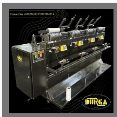
High speed automatic polyester yarn winder machine with digital counter meter
