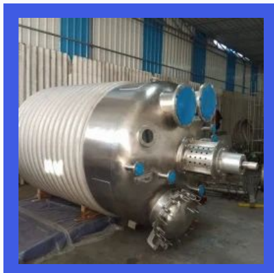
SS Reactor Vessel
